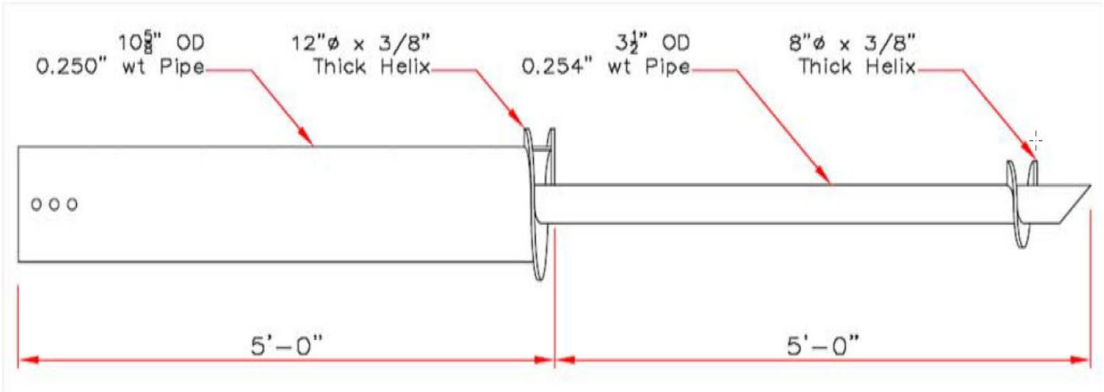
Soundwall foundation anchor drawing.
